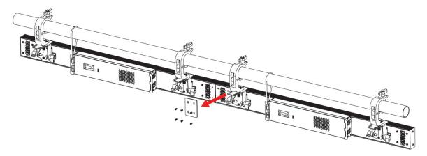
3. Place the connector plate across the gap between the two units, making sure to align the plate with the four (4) screw holes. Reinstall the four (4) screws that secure the connector plate in place, as well as the two (2) additional screws that held the connector plate in its storage position. The installation is now complete.
